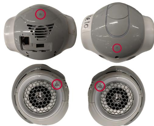
Figure 13. V4 and prior Nao robot microphone positions
