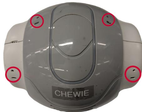
Figure 12. V5 and later Nao robot microphone positions
