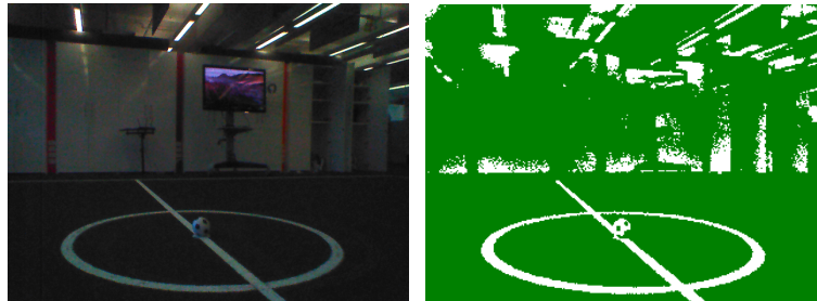
Fig. 3: An example of the adaptive thresholding process. White pixels are considered light whilst green pixels are dark.
